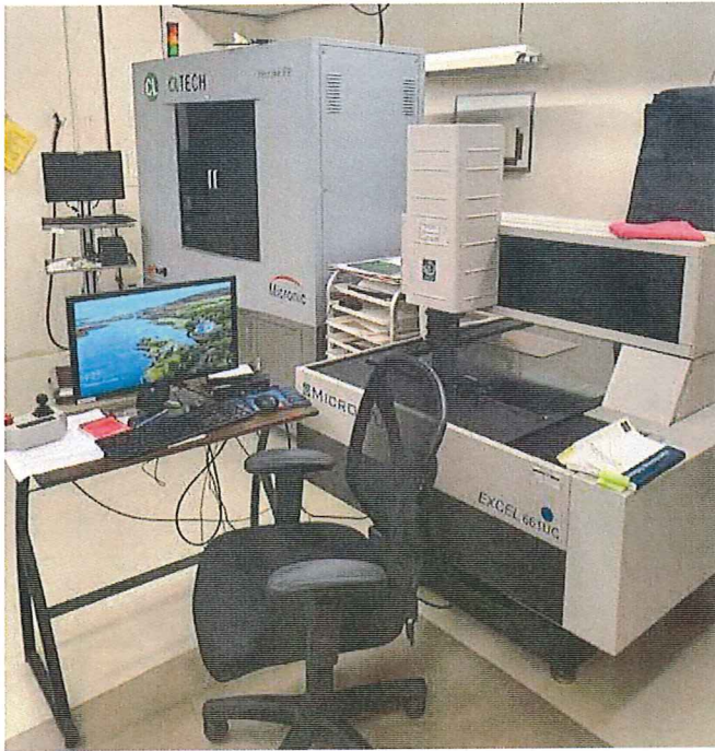
IMI's new purchase of a Micro-Vu Excel 661UC vision CMM has expanded their metrology capabilities in terms of accuracy, repeatability and speed.
